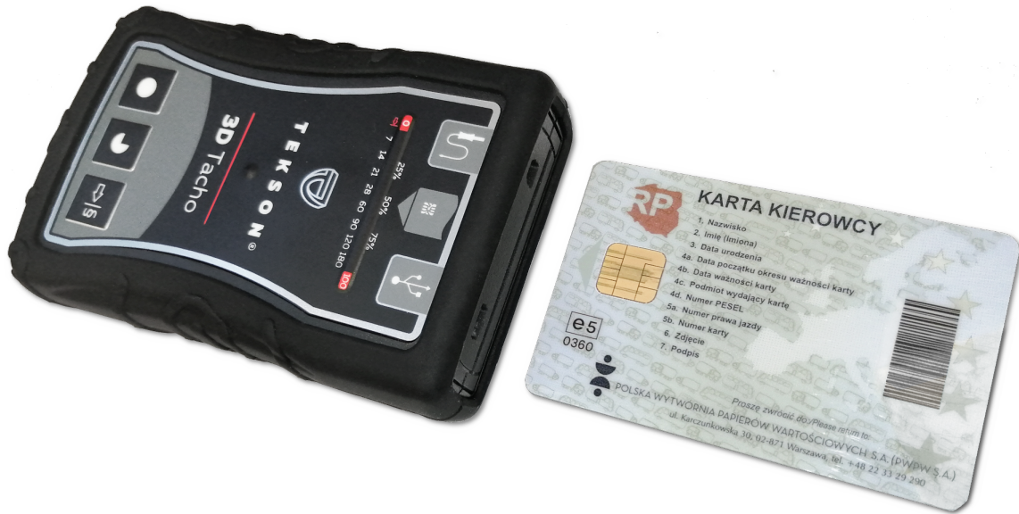
Fig. 3D Tacho - inserting a driver card.
